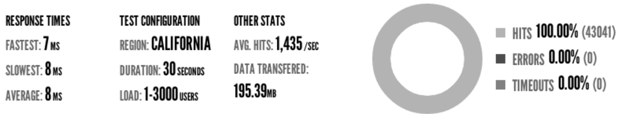
Figure 2: Blitz.io test results for Varnish powered Statamic, 43,041 successful hits in 30 seconds
