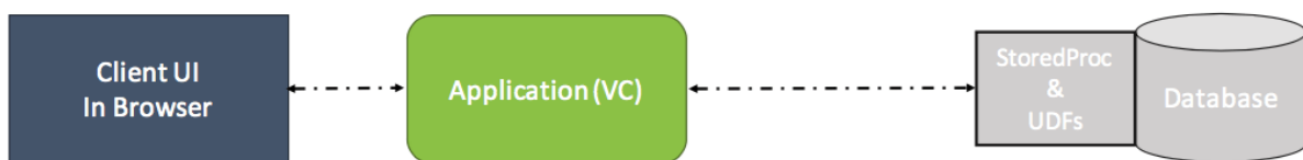
Figure 2: Executing stored procedures via an application to deliver data to a client UI in the browser. Quite similar to MVC application exception the Model layer i.e. M is missing
